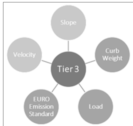
Figure 3 – Input Variables of the EMEP/EEA's HDV Tier 3 Approach
